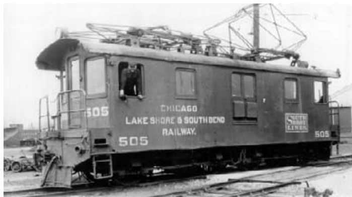
The Lake Shore had two freight locomotives which could handle up to 40 loaded cars each: one of them, the 505, is shown here on April 15, 1925, at the Shops in Michigan City. (Calvert's Studio photo, William Janssen Collection)
